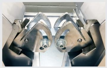
Easily adjustable safety guides allow polishing of a wide variety of cutting angles
